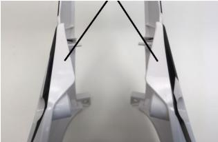
(VIEWING BOTTOM OF SHROUDS) Use a razor knife and a straight edge to score on dotted line. Remove templates. Trim shrouds.
